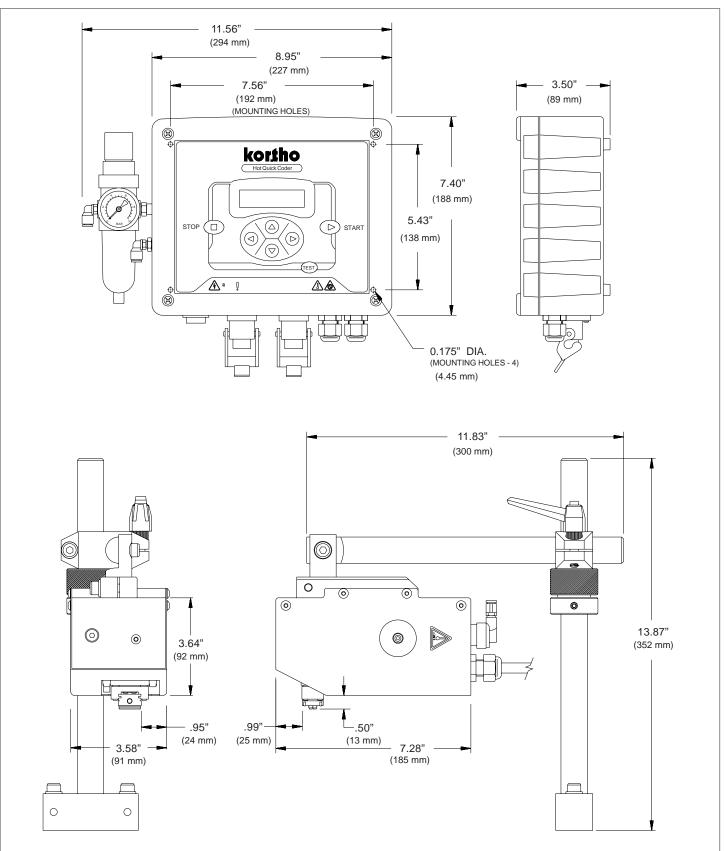
Print Area: Printing Speed Max: Product Speed Max: Working Pressure: 0.472" X 0.945" - (12 x 24 mm) 300 Prints/min. 196 Ft./min. - (60m/min.) 56 PSI - (4 bar) Electrical: Coder Weight: Control Weight: 110-130 VAC/1 A. 3.75 Lbs. - (1.7 Kg,) 4.41 Lbs. - (2 Kg.)
