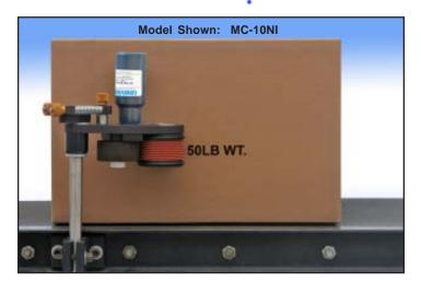
Universal's Reservoir Ink Cartridges plug right into the Mini-Coder for convenient, automatic re-inking of the ink roll during production. Standard models are supplied with Universal's RIBtype® die fastening system, a dry Microcell ink roll and an anodized aluminum mounting bracket.
