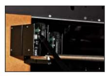
each module together which allows the hand held controller to network all of the print heads. The controller has the capability of controlling up to 32 individual print head modules. A longer cable is used to connect the
